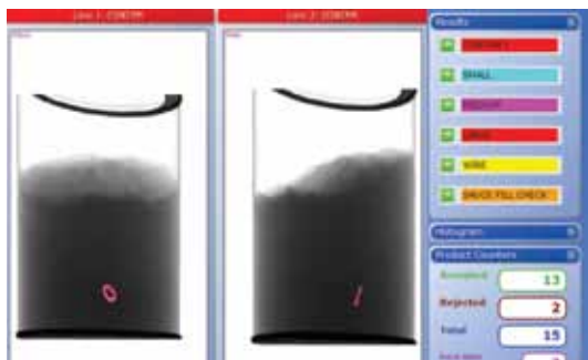
Figure 1: X-ray image of a contaminated can of milk powder
